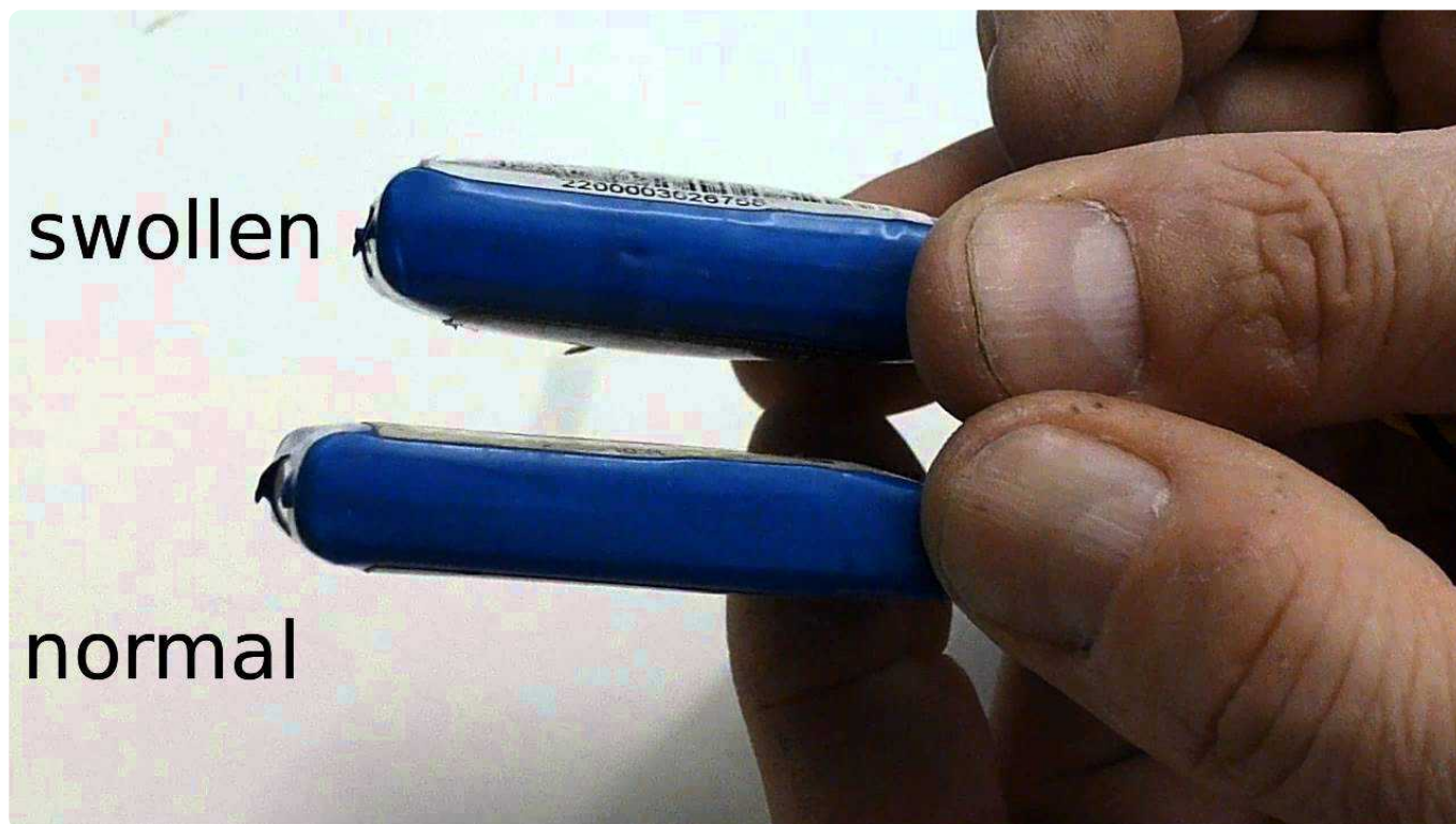
Example of a bulging LiPo battery pack that will need to be replaced.
